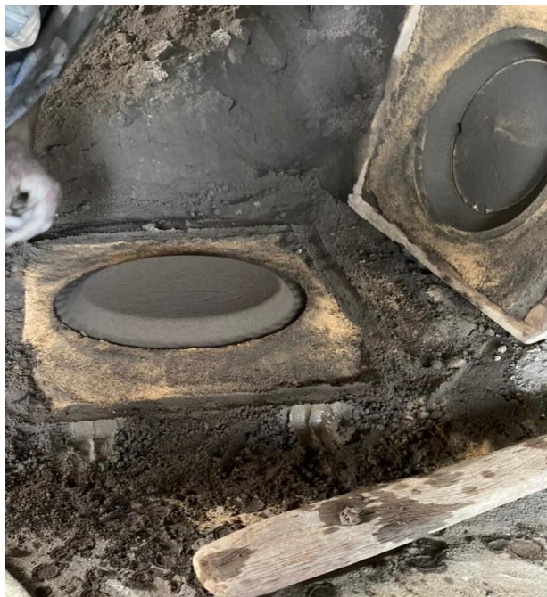
Figure 9. Mold to receive the molten aluminum
