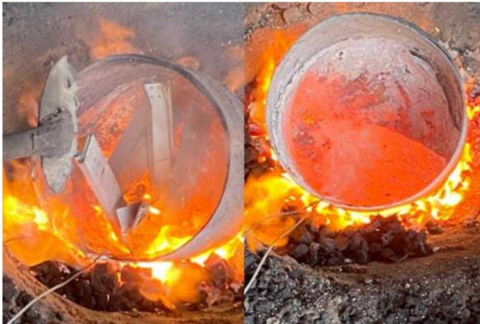
Figure7. Melting of aluminium: transition of aluminum from solid to liquid state
