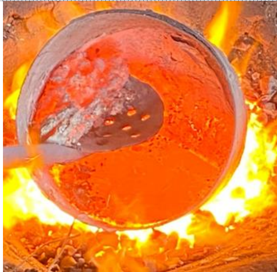
Figure 8. Removing impurities from aluminum
